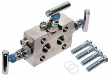
Direct mounted three-valve manifold, instrument mount to pipe connection. Offering two isolation valves, and one equalising valve for differential pressure transmitter or static instrument applications. Supplied with bolt pack and spare seals as standard. This slim, compact 3-valve manifold offers all the features of high integrity needle valve head design incorporated in one common instrument manifold block that mounts directly to an instrument.
